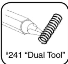
We include extra knuckle springs. To replace the knuckle spring, use our #241 Dual Tool (Manual Uncoupling Tool & Spring Pic) and insert it between the last two coils on either end of the spring. Then slip the end of the spring onto one of the retaining cones in the knuckle and compress the spring until you can slip the other end onto the opposing cone then withdraw the pick.
