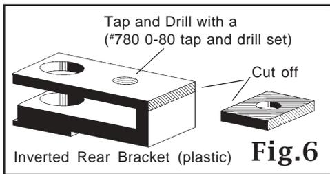
When mounting the replacement brackets to the chassis use the new flat springs and place the springs in their brackets first then slide the coupler/bracket assembly over the pivot hole and press the pin in firmly. Flip the bracket back and forth. If it does not 'snap' back
