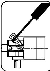
**NOTE:** To secure the knuckle spring more durably carefully dip the last two coils in DUCO® (or similar type of glue) or a thick slow drying CA glue ("do not" use the thin CA glue because it can easily "wick" into the knuckle and ruin the coupler). Then slip the end of the spring onto one of the retaining cones and compress the spring until you can slip the other end onto the opposing cone then withdraw the pick.
