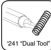
To replace the knuckle spring, use our #241 Dual Tool (Manual Uncoupling Tool & Spring Pic) and insert it between the last two coils on either end of the spring. Then slip the end of the spring onto one of the retaining cones and compress the spring until you can slip the other end onto the opposing cone then withdraw the pick.
