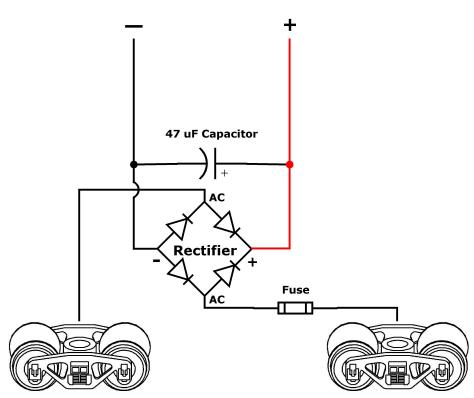
Kadee Rectifier Kit No. 169 converts AC or DC track current to polarized DC current suitable for LED lighting and other electronic devices that require DC current
