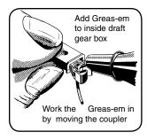
lid. The wire springs are quite resilient but not indestructible and are NOT REPLACEABLE so if you damage the spring the coupler can not be used again. When securing the lid or box cover make sure the coupler flexes back and forth freely.
