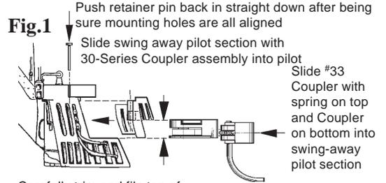
Carefully trim and file top of swing-away pilot section coupler opening to allow the 30-Series Draft Gear Box to slip fit in. Also be sure top of loco pilot opening is free of burrs and is flat.
