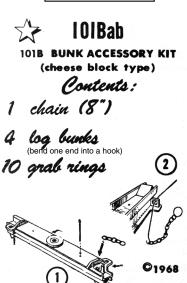
Kadee<sup>®</sup> Quality Products 673 Avenue C • White City, OR 97503 Suspend the chain between the two pins stuck into a board. Count 15 loops from the end and clamp in a grab ring. Count 16 loops and clamp in another grab ring; do this two more times. Now cut the loop just behind each grab ring, and you will have four chains of 15 loops, with a grab ring on the last loop.
