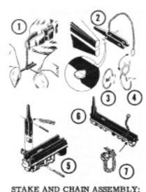
A piece of chain 1 7/8" long is attached to each stake, this can be accomplished by suspending chain from fixed position so that one end will hang free, leaving both hands available for attachment. Fig. 1 shows one satisfactory method. A small clamp
