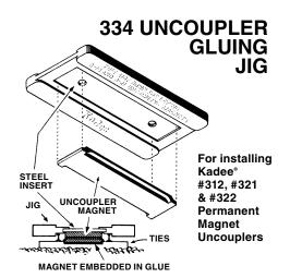
This jig removes all guesswork when installing Kadee® permanent magnet uncouplers... assures magnet will be permanently centered in the track at the absolute recommended height for optimum performance!
