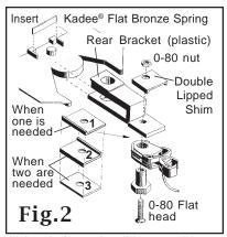
with the smaller double lipped shim on top of the platform followed by the 0-80 hex nut and tighten snugly. If the assembly turns on the bracket after the screw is tightened you may have to use a very small drop of CA cement between the shims and the bracket or where it is needed. This option can use any combination of the die cast shims to achieve the correct coupler height.
