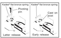
over the post capturing the spring. Flip the bracket back and forth to check for free movement then check for the correct coupler height. Make any necessary adjustments.
