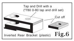
When mounting the replacement brackets to the chassis use the new flat springs and place the springs in their brackets first then slide the coupler/bracket assembly over the pivot hole and press the pin in firmly. Flip the bracket back and forth. If it does not 'snap' back
