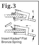
Check and make sure that the length of the coupler reaches out enough to clear both pilots. You may have to move the hole in the bracket a little forward or retain the original bracket conversion. For the rear of the 'A' unit use option #1 as above but with the short shanked coupler (#33) and the spring side of the draft gear box on the bottom of the coupler.
