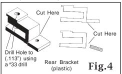
with the #36 long shanked coupler and the spring side of the gear box on the bottom. Also use option #2 but with the #33 short shanked coupler for the rear of the E-7 'A', PA, and both ends of the later production E-7 'B' unit, with the spring side of the gear box on the bottom.
