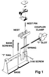
clamps coupler knuckle. Caution: Do not allow fixture clamp to snap forward. Assemble centering spring into coupler shank and lid onto draft gear box according to coupler instructions.
