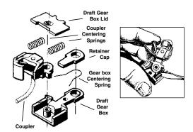
To assemble the coupler follow the illustrations in these instructions. Secured lid to the gearbox with the #2 x 3/8" screw. Add a "puff" of our #231 Greas-em into the draft gear box. Make sure the coupler flexes back and forth freely.
