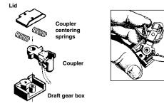
To assemble the coupler follow the illustrations in these instructions. The gear box lid is not secured with the screw until it is mounted. Add a "puff" of our #231 Greas-em into the draft gear box. Make sure the coupler flexes back and forth freely.
