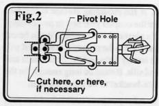
3. Turn the car over and position the coupler gear box assembly with the flex-bracket where it will be located (Fig.1). Check for clearances and decide which two of the four mounting holes on the flex-bracket are best suited for your application. You may need to cut off the two side tabs or rear tab for added clearance (Fig.2).
