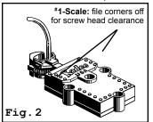
position, slightly file raised surfaces inside of bracket.) Now place the other 2 x 3/8" screw in rear mounting hole (replacing Screw B). DO NOT over tighten this screw.
