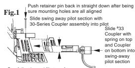
Carefully trim and file top of swing-away pilot section coupler opening to allow the 30-Series Draft Gear Box to slip fit in. Also be sure top of loco pilot opening is free of burrs and is flat.
