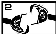
2 Withdraw slightly to disengage couplers. Magnetic force of the uncoupler draws couplers apart, uncoupling them.
