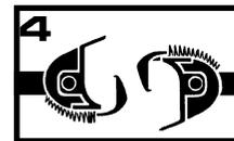
4 Withdraw, leaving uncoupled car(s) on desired track. Couplers automatically return to normal coupling position.
