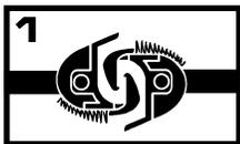
1 Stop over a Magnetic uncoupler, allowing slack to occur between the couplers. Knuckles have opened.
