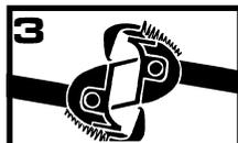
3 Enter over uncoupler again, couplers are in delayed position allowing pushing of car(s) without causing re-coupling.
