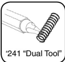
NOTE: To secure the knuckle spring more durably carefully dip the last two coils in DUCO® (or similar type of glue) or a thick slow drying CA glue (“do not” use the thin CA glue because it can easily “wick” into the knuckle and ruin the coupler). Then slip the end of the spring onto one of the retaining cones in the knuckle and compress the spring until you can slip the other end onto the opposing cone then withdraw the pick.
